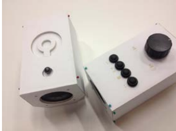
Figure 2. Semantic interactive prototype on the left, function is activated by tilting or metal ball. Conventional prototype with buttons on the right.
