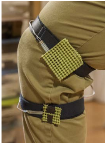
Figure 5 (top) & 6. The top photo shows the hardware components that attach to the outside of the leg (ESP, ERM, battery) and the bottom photo shows the FSR location on the inside of the leg.
