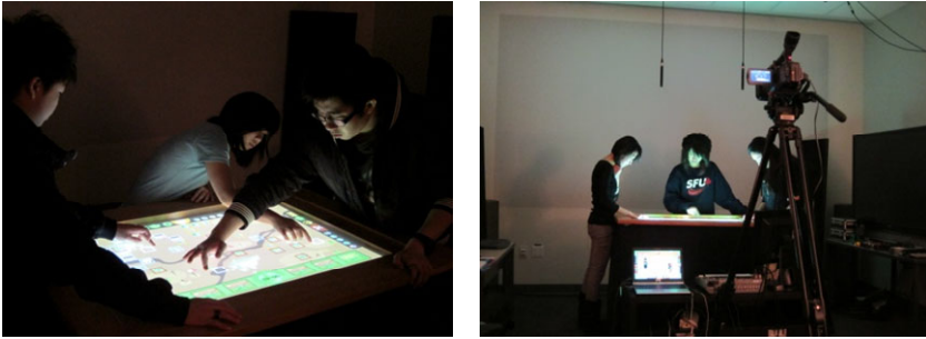
Fig. 4. Playing Futura in groups of three (left). The setup of the user study, showing the Futura game tabletop, three players, microphones, video camera and a additional screen (right).
