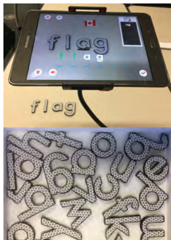
Figure 2: The AR PhonoBlocks system: a tablet running an AR app and a set of magnetic physical letters with black markers.
