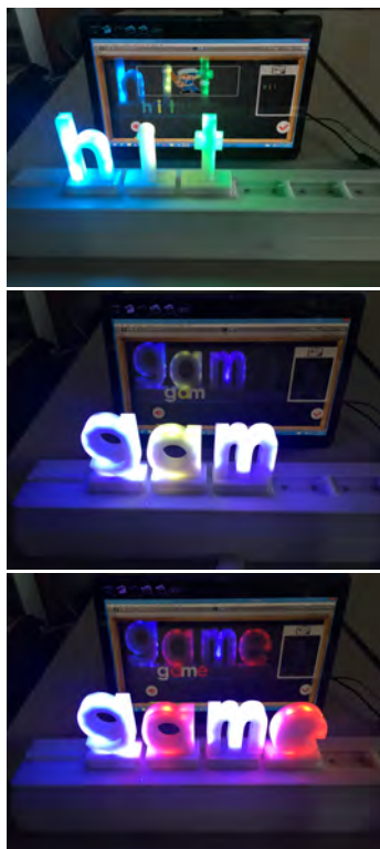
Figure 1: PhonoBlocks contains a touch based laptop, a customized platform and a set of tangible letters with LED lights ( up ). LED strips change colours to indicate letter sound change. In the Magic-e Rule, the colour a changes from yellow to red to indicate sound change from short to long ( middle and down ).
