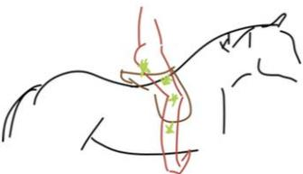
**Figure 2.** A side view of the areas of the 'seat' used to gather pressure data as well as provide site-specific vibrotactile feedback. At these points, pressure (FSR) sensors will be mounted on the inside of a rider's leg and the vibration (ERM) motors will be mounted to the outside.
