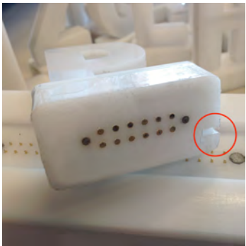
Figure 3. The magnetic notch on each letter and openings in each slot utilizes physical constraints to enforce correct orientation of each letter in its slot.
