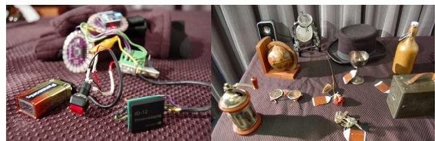
**Figure 1. The components of the glove: Arduino Lilypads, XBee radio & RFID reader**
