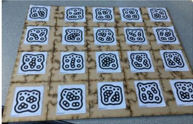
**Figure 3:** Each piece has a unique fiducial marker pattern.
